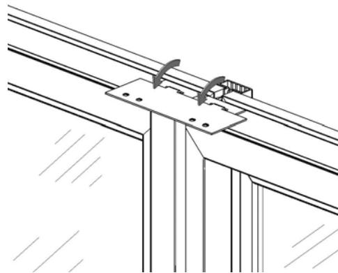
2. Follow the procedures listed on the installation instructions for the particular windows being installed. Lift the windows, with the mullions and base plates attached, into the opening. Make sure the entire unit is plumb, level, and square.
